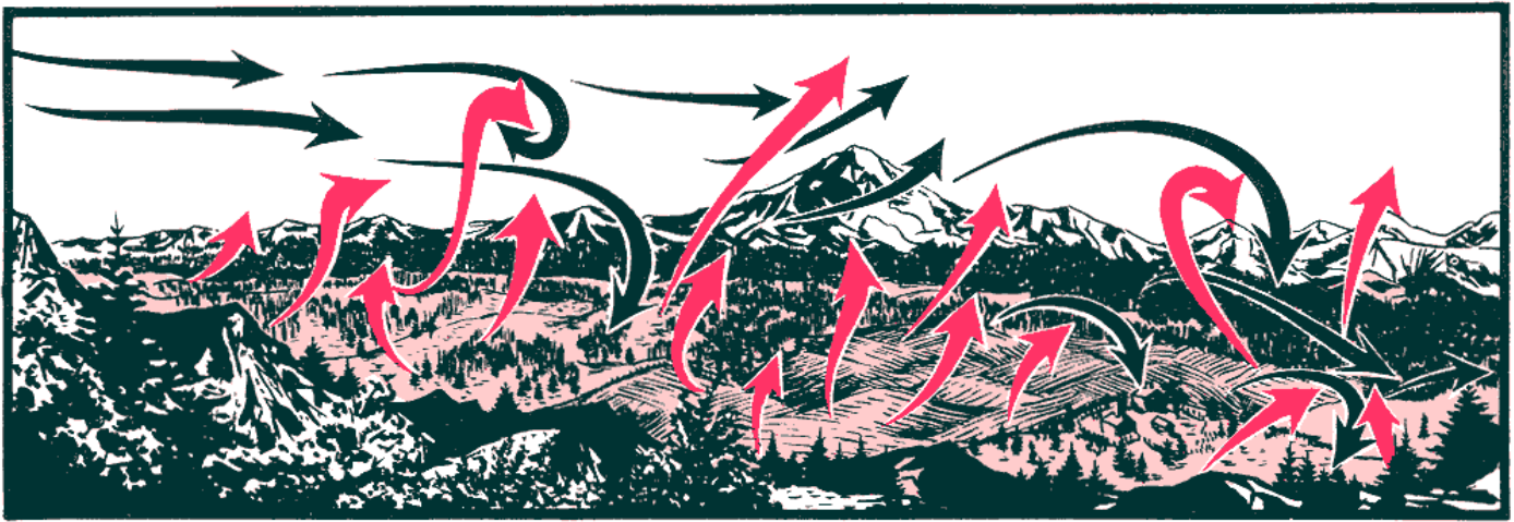
Thermal turbulence caused by surface heating is a mechanism by which energy is exchanged between the surface and the flow aloft. This mixing brings higher wind speeds from aloft down to the surface, usually in spurts and gusts.
